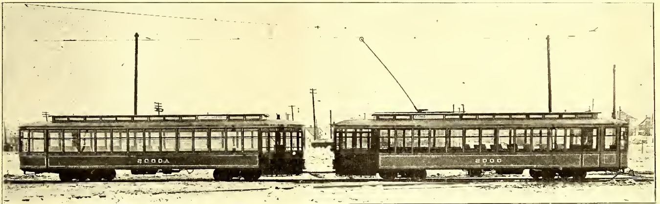
UNIT OF TWO LOW-FLOOR CARS BEING TRIED OUT ON TWIN CITY LINES
